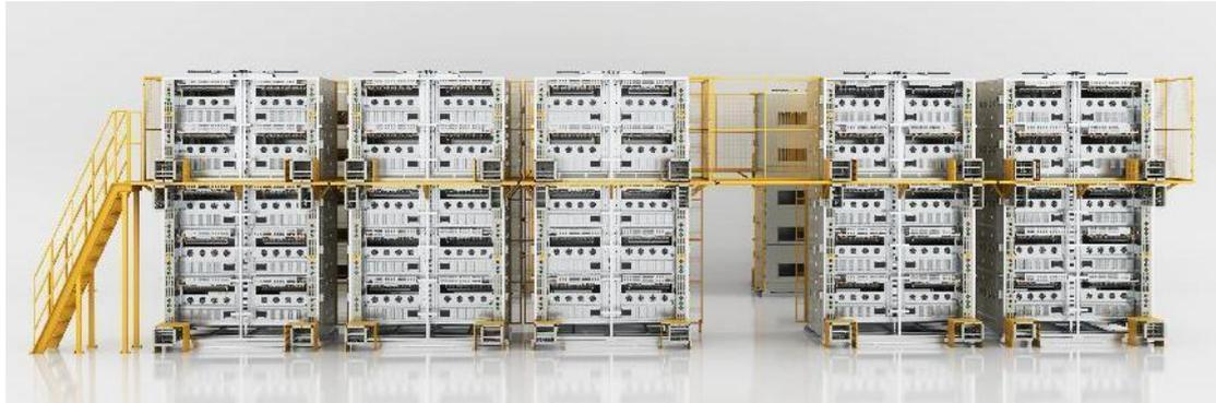
Negative pressure formation chamber adopts a six-sided protection design. It is equipped with dual fire protection (water & gas).
